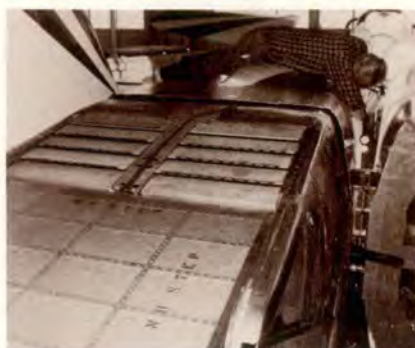
A technician checks the thrust vectoring nozzles prior to flight. Their operation is transparent to the pilot. That is, they respond entirely to inputs of a computer.
