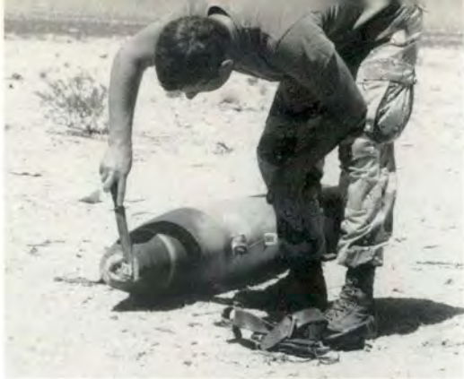
MSgt Costlow inspects the fuse of one of many MK-82 500-pound bombs which impacted before it had armed.
