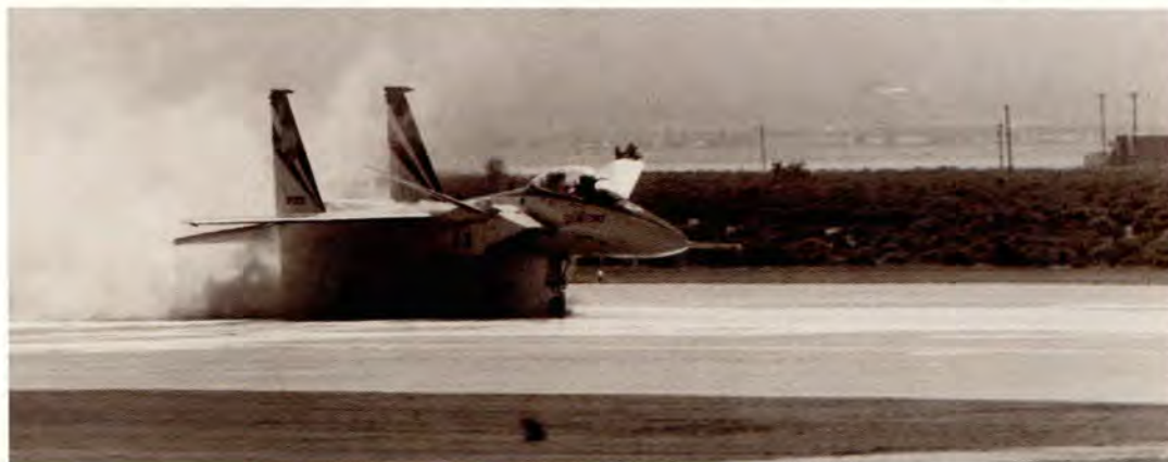
The extensive testing of the F-15 STOL/MTD includes short field landings on flooded runways.
